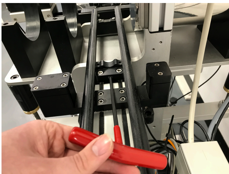
Figure 3.2: Rail sleeper removal bolt
