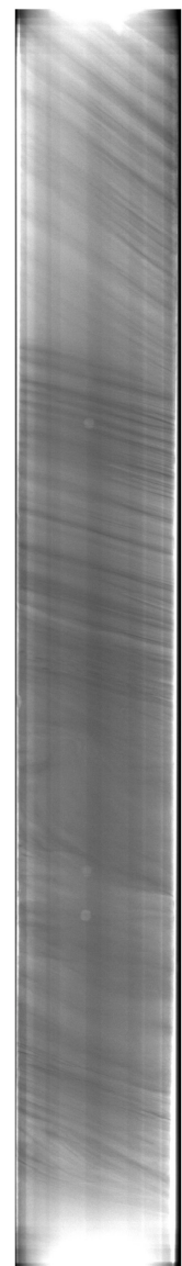
X-ray Radiograph of 1m Whole 4" Aluminium Lined Rock Core
